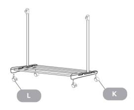
**Note:** All metal tubing must be securely inserted into the plastic parts and connectors to ensure proper assembly.
