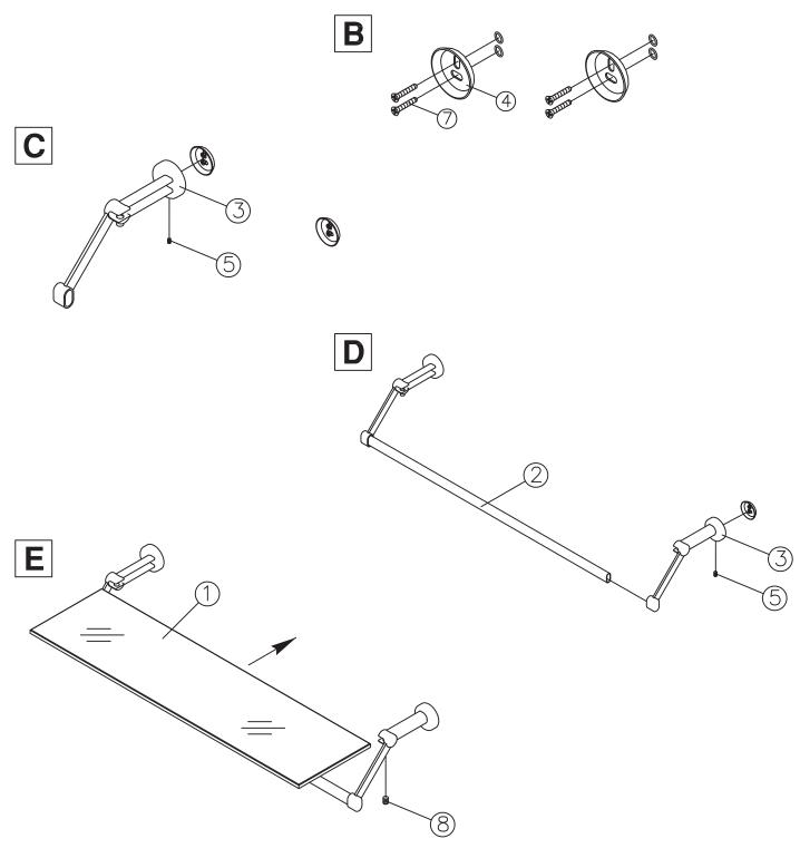
Please note: Part #8 (screw) should be loosened from part #3 (hinges) first before placing the glass shelf on hinges. After glass is settled, part #8 screws may now be tightened.
